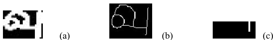
Fig. 7. Example of Class-2 normalisation. (a) Class-2 symbol, (b) Normalized symbol; (c) segment-2 extension separated
