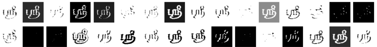
Fig. 4: Total 32 features or the responses of filters at the output of first convolution layer.
